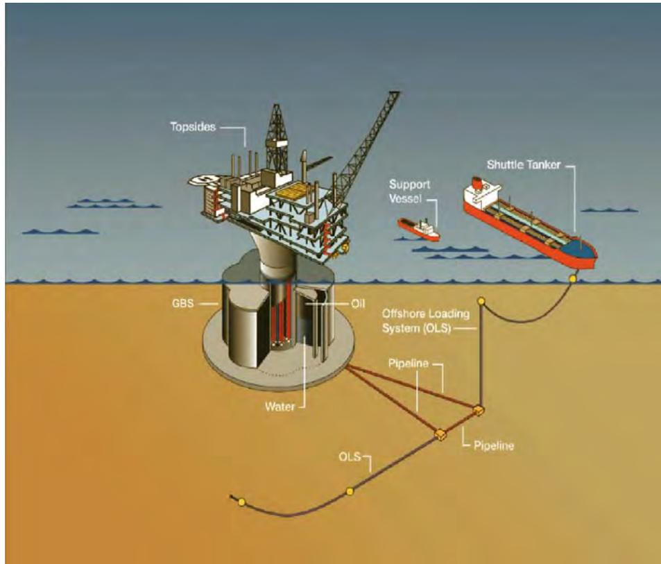
**Figure 2-5 Stand-alone Gravity Base Structure Preliminary Development Layout**
