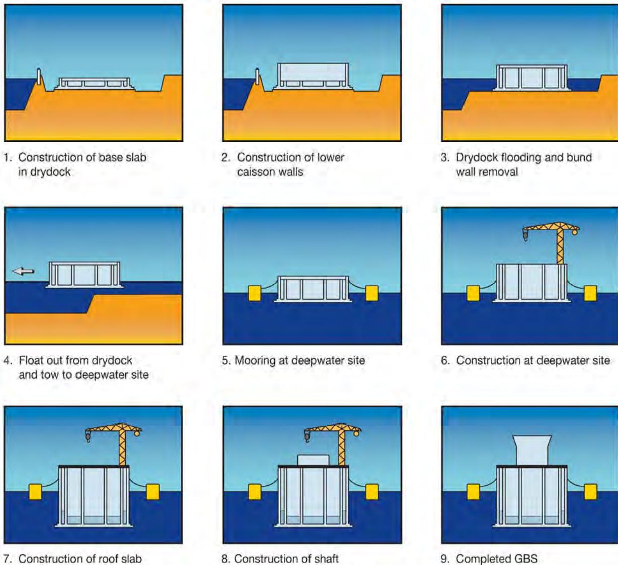
**Figure 2-11 Schematic of Building a Gravity Base Structure**
